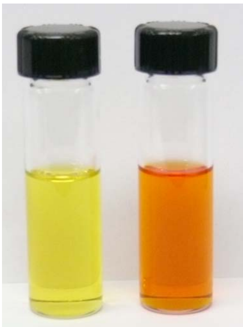
Figure 1. Solutions of copolymer 4 in \text{CH}_2\text{Cl}_2 (left) and after exposure to TBAF (right).
